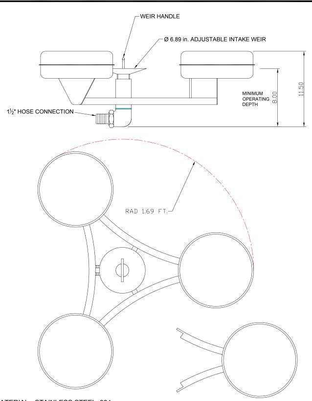
MATERIAL - STAINLESS STEEL 304 WEIGHT - 19.8 Lb. SUPPLIED WITH 10 FT. SUCTION HOSE & COUPLINGS ALL DIMENSIONS IN INCHES UNLESS STATED
