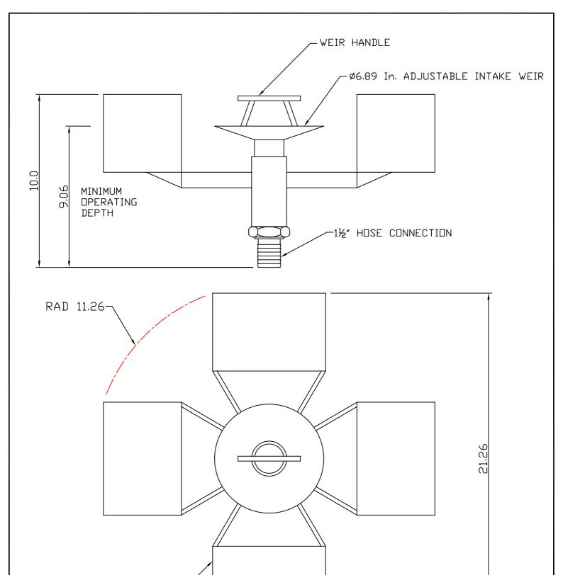
MATERIAL - STAINLESS STEEL 304 WEIGHT - 22 Lb. SUPPLIED WITH 10 FT SUCTION HOSE & COUPLINGS ALL DIMENSIONS IN INCHES UNLESS STATED
