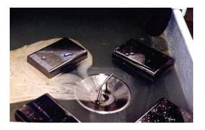
Using the appropriate weir setting, Megator skimmers will deal equally well with thin surface layers of light oil or concentration of heavy oils.
