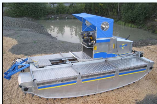
The movable driver's cab is hydraulically adjusted and works as a counter-weight during heavy lifts in water.
