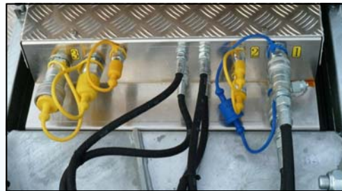
Hydraulic outlet for operation of tools; regulated using a joystick on/off and max/min rpm of the tools.
