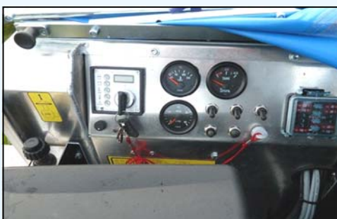
The instruments show hydraulic pressure, fuel level, motor temperature, hydraulic oil temperature, a chronometer and the motor revolutions as well. Track speed is easily regulated by turning a knob.
