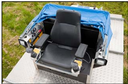
Ergonomic driver's seat with joysticks for regulation of steering, speed and tools.
