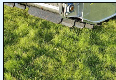
The low weight gives a low ground pressure. Truxor can be driven on a lawn without damaging the grass.
