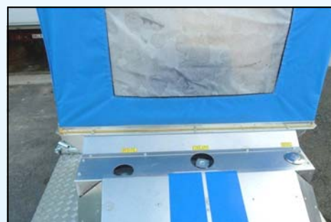
Easy-to-access diesel tank and a hydraulic oil tank for the control and refilling of fluids.
