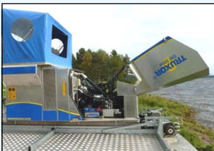
The engine cover is opened as shown. A tool box is located inside the engine compartment.
