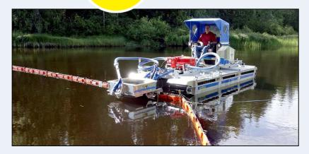
Doro Skimmer DS 800 is a combi-skimmer that works mobile and in shallow waters from approximately 0.8 in. water depth. When oil spill have been contained with oil booms, the boom can be attached to the skimmer. This keeps the machine from driving in the oil spill. The gables of the Doro Skimmer can be disassembled, this increases the capacity if the oil is thicker.
