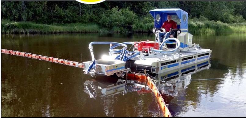
**Doro Skimmer DS 800** is a combi-skimmer that works mobile and in shallow waters from approximately 0.8 in. water depth. When oil spill have been contained with oil booms, the boom can be attached to the skimmer. This keeps the machine from driving in the oil spill. The gables of the Doro Skimmer can be disassembled, this increases the capacity if the oil is thicker.
