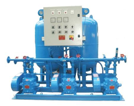
**Megator marine pressure sets** are compact self-contained units, incorporating the highly successful sliding-shoe pumps, hydraulic accumulator, inter-wired control panel and all interconnecting piping assembled on a fabricated steel frame. On-board installation only requires piping connections to suction and discharge manifolds, connection of main electrical supply to control panel.
