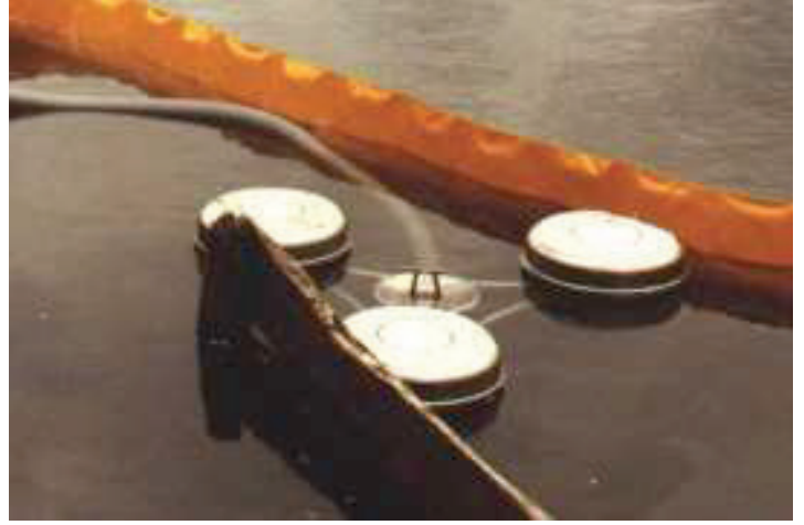
▲ Preventing floating debris from clogging the skimmer on a pond.
